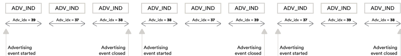
Figure 5 - Advertising channel use per the Bluetooth Core Specification 5.1 with a randomized channel index sequence
